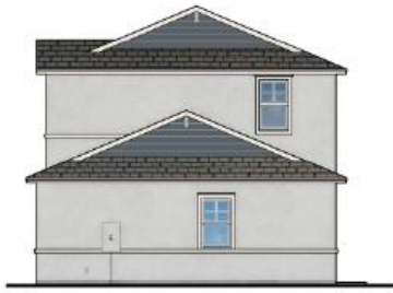
RIGHT ELEVATION ELEVATION C 1/8" = 1'-0"
