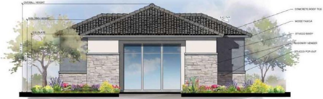
FRONT ELEVATION ELEVATION B 1/8" = 1'-0"
